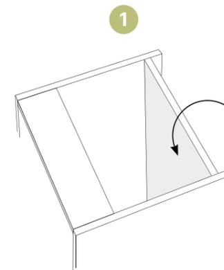
18mm back panel for added rigidity on base units, means you don't need to worry about your cookware damaging the backs!
