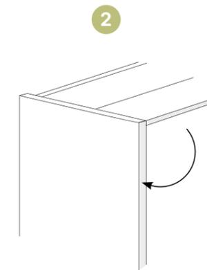
2mm PVC on leading edges prevents moisture from getting into the cabinet structure and causing damage.
